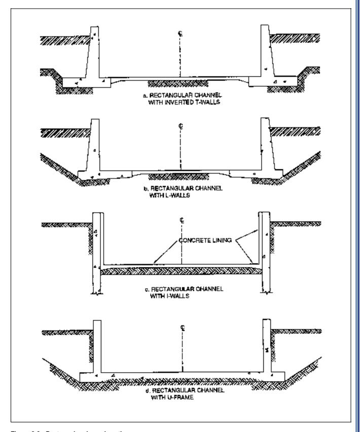
Figure 2-2. Rectangular channel sections
