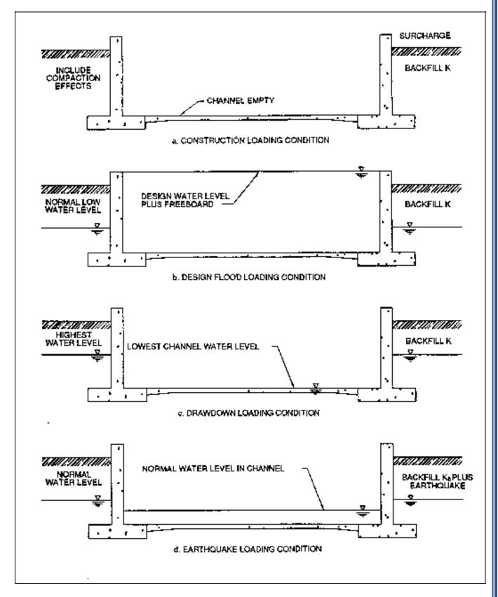
Figure 4-1. Loading conditions, rectangular channels with retaining walls
