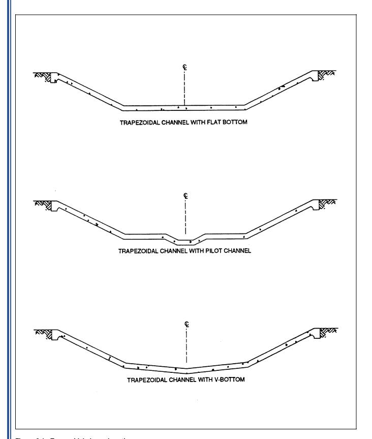
Figure 2-1. Trapezoidal channel sections
