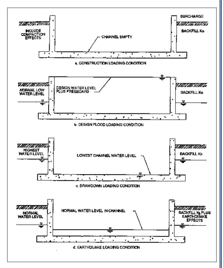
Figure 5-1. Loading conditions - rectangular channels with U-frames
