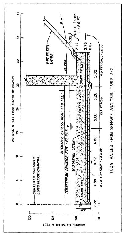
Figure C-7. Flows into drainage blanket from analysis of U-frame channel section
