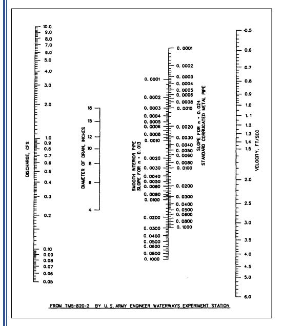
Figure C-9. Airfield drainage nomograph for computing required size of circular drain, flowing full
